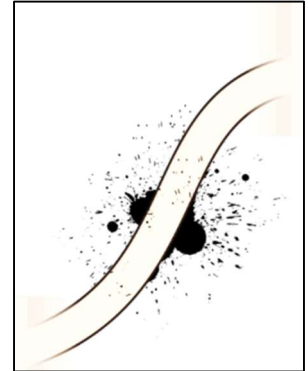
Visible signs of corrosion which may suggest pinhole breaks in sheathing
