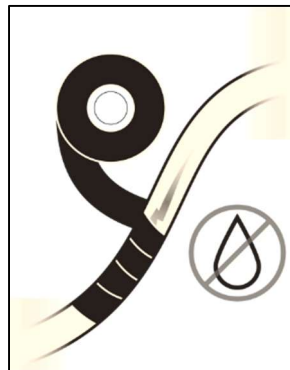
If cable sheathing is damaged but no internal damage is found, use seal tape on areas with damage to prevent moisture ingress.
