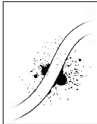
Visible signs of corrosion which may suggest pinhole breaks in sheathing
