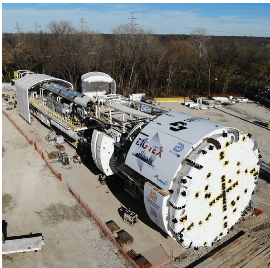
The project will provide 100-year flood relief for 2,200 commercial and residential properties. Here, the "Big Tex" TBM is assembled above ground in preparation for deployment.
